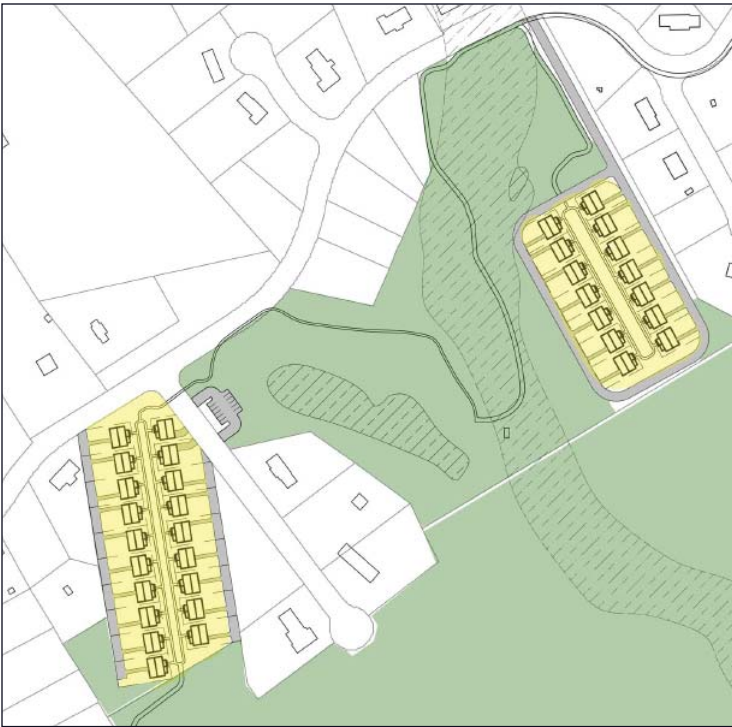
Study of Laurel Ridge area showing single-family houses fronting on a green and accessed via a rear-access lane.
