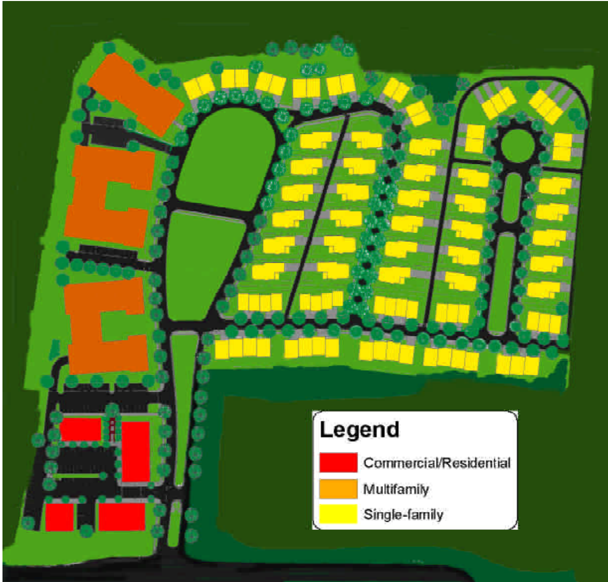
Site Plan of Colonial Green, a housing cluster currently being developed off of Colonial Avenue. This site plan illustrates how a large number and variety of housing units can be developed with commercial buildings and landscaping while retaining green space.
